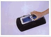
Remove the coated bridge from the plastic bag, touching only the raised lugs. Give the bridge a final shake to remove excess powder. Clip the bridge onto the base and wipe the base free of powder.
