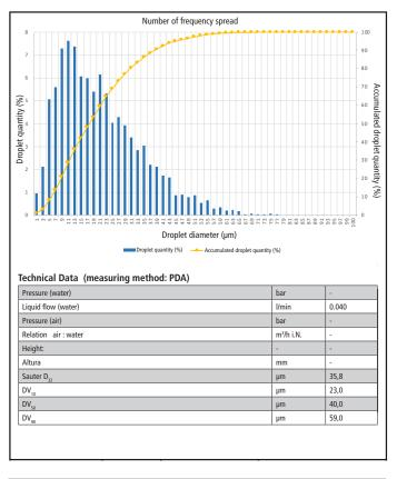
MND = NMD (number median diameter). Half of the droplet quantity is smaller , half is bigger than 19  $\mu$ m.
